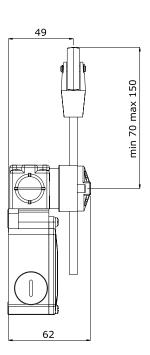
Standard limit switches are equipped with 1NO+1NC snap action switches PRSL0036XX  $\begin{bmatrix} 1 & 21 \\ 14 & 22 \end{bmatrix}$
